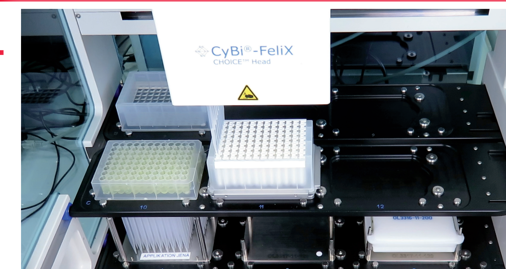
Fig. 1 | Fully automated handling of scienova Xpress Micro Dialyzer with Analytik Jena's liquid handling device Cybio® FeliX.
