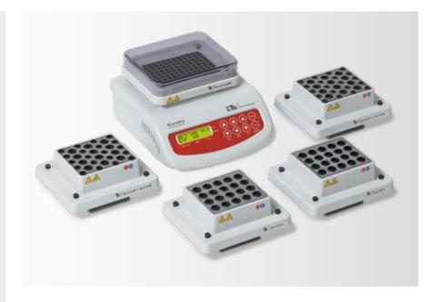
The Biometra TSC ThermoShaker is a thermomixer with heating and cooling function, as well with a variable mixing speed from 250 rpm to 1,400 rpm. Active cooling with Peltier technology allows a temperature adjustment from  $+4 \,^{\circ}\text{C}$  to  $+100 \,^{\circ}\text{C}$ .
